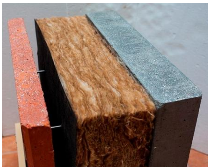
Slika 24 ECO-SANDWICH - predgotovljeni sendvič panel (ECO-SANDWICH, 2015)
